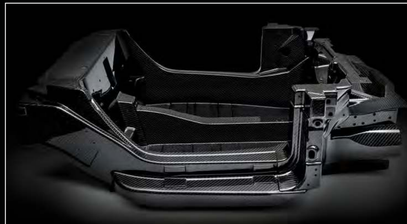
Genuine carbon fiber monocoque chassis
