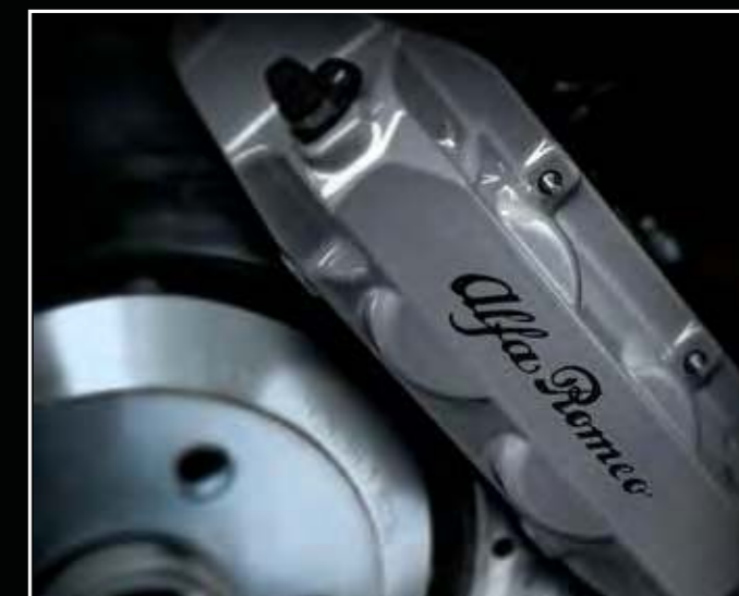
Dual-cast, perforated, self-ventilated, 305 x 28-mm front discs with Brembo® fixed 4-piston calipers
