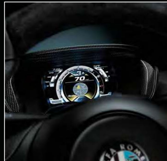
Full-digital instrument cluster with Thin Film Transistor (TFT) display and carbon fiber cluster surround
